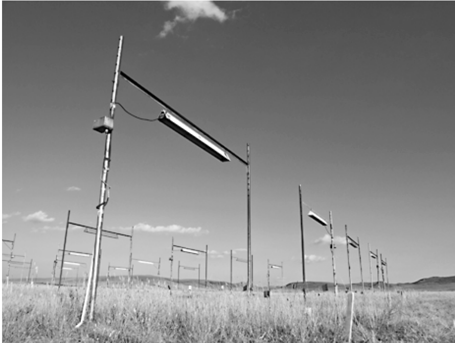
PLATE 1. Infrared heaters to conduct day (6:00 a.m.–6:00 p.m.), night (6:00 p.m.–6:00 a.m.), and diurnal (24 hours) warming in a temperate steppe in northern China. Photo credit: J. Xia.
